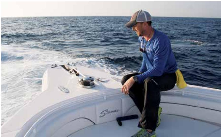
**Above: Vargas mans the Quick free-fall windlass on the 392 while anchoring up to fish a wreck in 150 feet of water. Right: The rigging station includes tackle storage, freshwater, sink, fridge and grill.**
